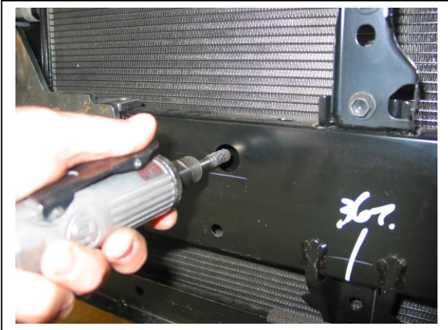
Figure 3: Enlarge centre holes to enable access for 3/8 nuts on wire
