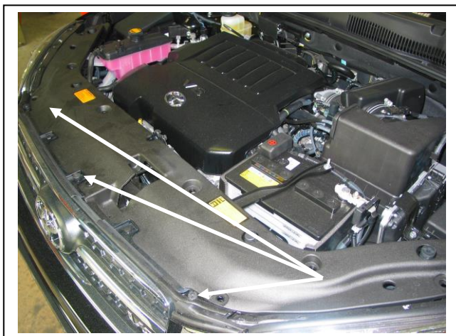
Figure 1: Positioning of bonnet rubber clip and screws
