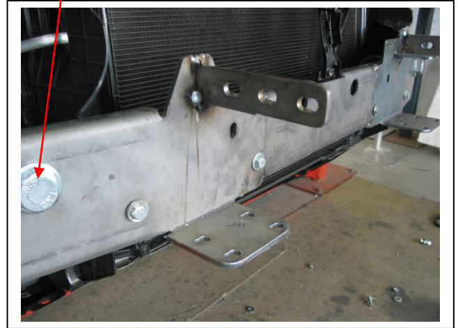
Figure 4: ECB steel mounting bracket fitted to vehicle.
